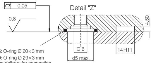
RSX3 - RSX6: O-ring  $\varnothing 20 \times 3$  mm
