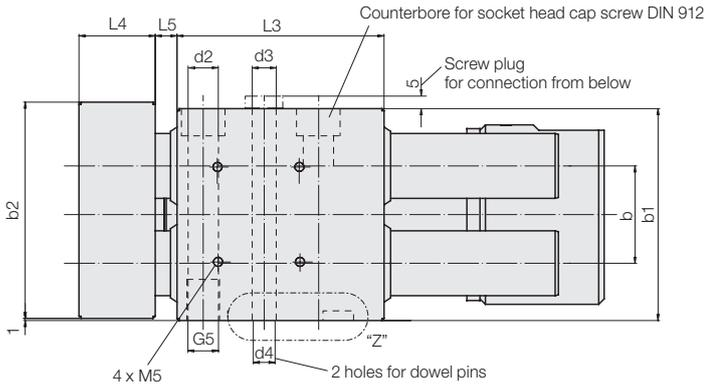
Connecting dimension for manifold-mounting connection and keyway
