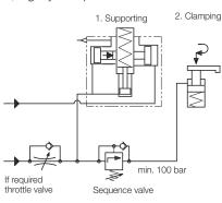
The sequence valve has to be adjusted to an opening pressure above the intersection of the two straight lines in the diagram.
