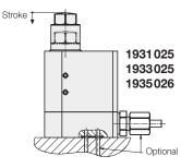
When loading the fixture, the support plunger is pushed back by the workpiece and makes contact with the workpiece by spring force. Hydraulic locking can then be initiated. During unclamping the support plunger will be unlocked and extends with spring force when the workpiece is removed.
