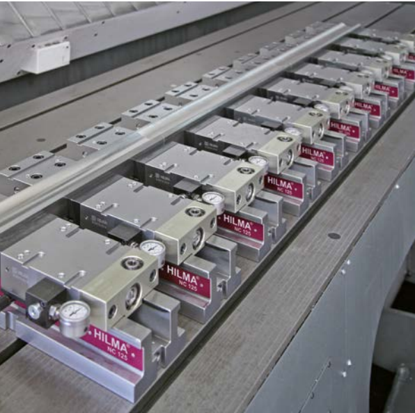
HILMA.NC with clamping force display
